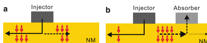
Fig. 6 Schematic illustrations of the flow of the spin current in (a) single F/N junction and (b) an F/N junction with an F contact
